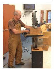
Gene's demo used a 6"x6" block of solid redwood. To start the box, Gene cut off a %" back slice. Gene prefers to cut the back off the rectangular blank first. He likes that this provides a flat back for cutting the profile. He cuts the back off and marks it to make sure he can align the pieces correctly later for reassembly. Gene then cut out the outside profile of the box by following the pencil line he created from his template. (There was a suggestion from audience to chamfer the back edges
