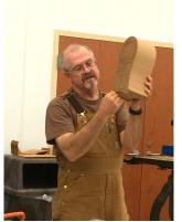
The grain in this blank is vertical, so Gene makes the entry cuts for the drawers vertically at one corner of the opening so that the re-glued cut is less visible in the grain. He enters from the bottom and cuts up one side to the top drawer first. He then works down the blank to the 2nd and 3rd (lowest) drawer in order, not pausing to remove the drawer blanks. Gene uses the lines on his blank for drawer outlines as "suggestions" - it is essentially a freeform cutting process.
