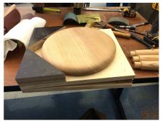
Tim uses an angled jig on his drill press to hold the seat blank at the proper angle for the legs. The jig tilts the seat at an angle of a few degrees from horizontal, which allows the leg mortises to be drilled at a uniform angle. Tim just used guesswork last night to set the angles, but if he had it to do over, he would have picked a higher angle to provide more leg splay than used on the demonstration stool.
