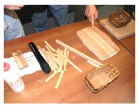
When attaching the pattern, be sure to allow time for the spray adhesive to become tacky. This takes several seconds. Do not just spray and immediately attach to the wood because this will make a permanent bond. Attach the pattern as flat as possible.
